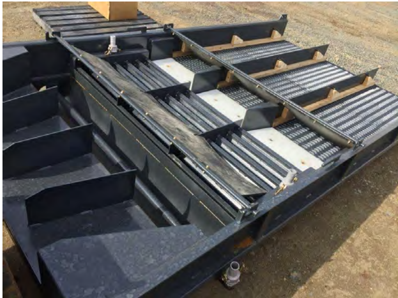
Fig. 1 – Hydraulic Riffles followed by expanded metal
