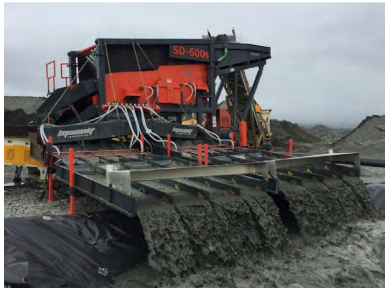
Fig 2 – Water distribution lines providing filtered water to hydraulic riffles
