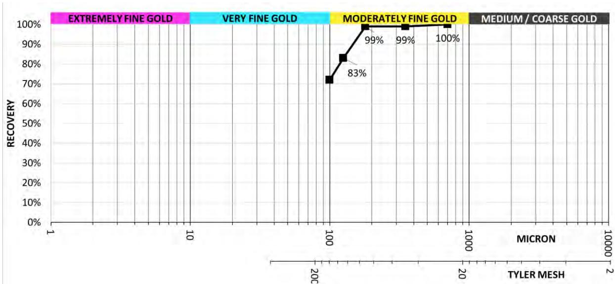
The recovery curve is constructed from gold in concentrate (measured in the field) and gold in tailings (measured by laboratory).
