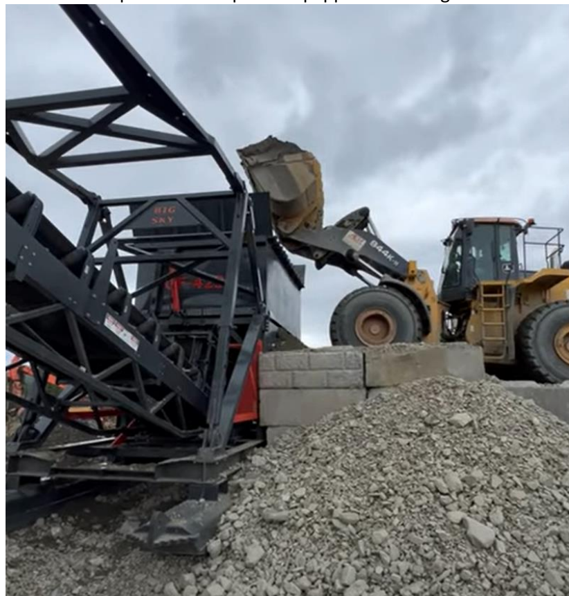
Fig. 2 – Paygravels hauled and fed by Front End Loader into Grizzly Feeder
